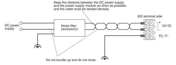
\* Noise filter is not required for controller unit hardware version "03" or later. Noise filter is not attached as accessory with above version.
